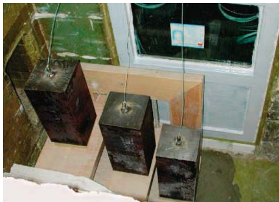
Hot and heavy. This Fraunhofer Institute test furnace measures how much weight treated wood can bear after burning.
